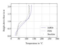
Temperature profile (at the bottom) at the center of the doorway
